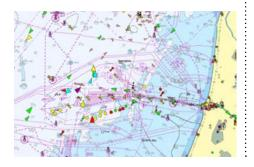
Bridge systems today permit AIS data to be overlaid onto radar screens and in many cases electronic chart displays. Successful operators use their Management of Change Policies to manage the potential for importation of risk with new technologies, but it is becoming apparent that AIS-assisted collisions are on the rise.
