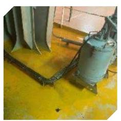
Hydraulic fluid accumulated in steering gear saveall
