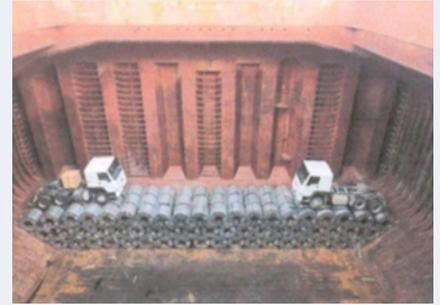
A five-hold geared bulk carrier loaded mixed stowage of bagged cargo, vehicles and steel products at China for offloading at Africa and Brazil. The Charterers' Pre-Stowage Plan had indicated to the Master that bagged cargo, vehicles and steel bars were planned to be loaded above steel coils. The Master did not raise any protest at this pre-stowage phase.
