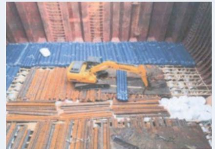
The loading progressed despite the Master's concerns with vehicles loaded atop the bagged cargoes, shown below.
