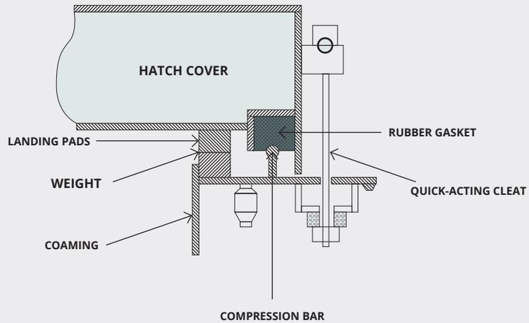
Heavier hatch covers led to landing pads being developed to take the weight. These also had the effect of improving weight transferral of any hatch top deck cargo into the ship's hull.
