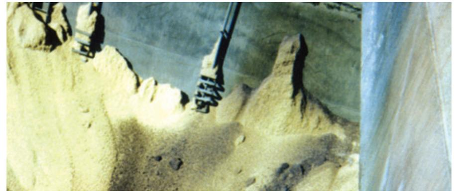
✓ Take precautions if loading sensitive cargo against heated bulkheads, bunker tanks or engine room.
