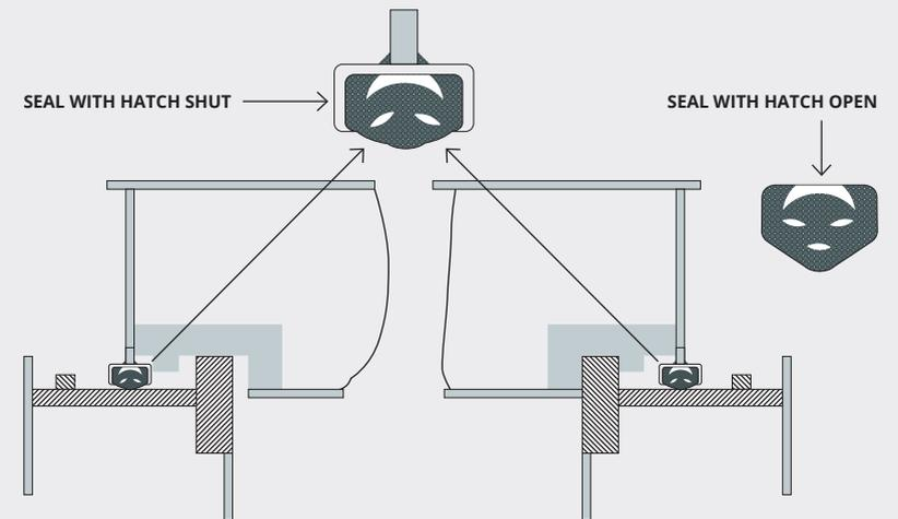
Compression bars made of highly corrosion-resistant material were introduced to reduce ongoing maintenance to both the bars themselves and also the sealing rubbers. The extra initial cost is many times cheaper than subsequent replacement parts and labour, not to mention the reduced potential for cargo claims.
