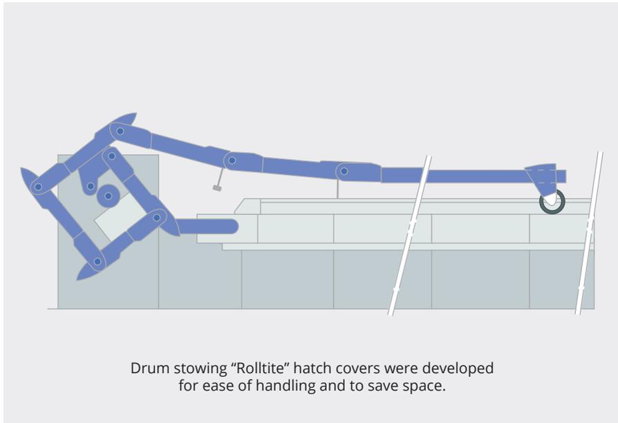
Drum stowing "Rolltite" hatch covers were developed for ease of handling and to save space.
