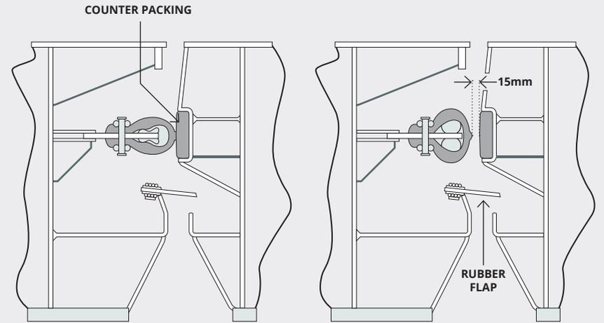
Sliding rubber systems do not use compression bars and allow greater movement between coaming and hatch cover. The Omega sealing system is shown above with the Cat sealing system shown below.
