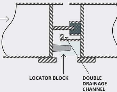
Double drainage is important to lead minor leakage away through the drain valves and is an essential component in the weathertight integrity system.
