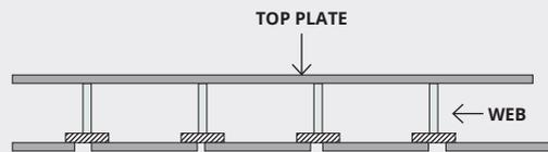
Double-skinned or box type covers were developed to span large openings. They provide equivalent strength to those with open construction without protruding so far down into the cargo space and losing cargo-carrying capacity.
