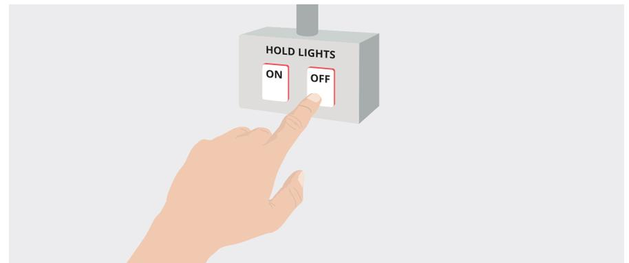
✓ Ensure hold lighting is switched off when not in use and remove fuses on a laden passage.
