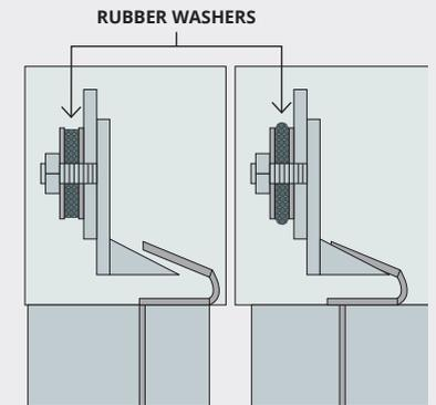
The reduction in crew necessitated less labour-intensive securing arrangements and the auto-cleat system was developed.
