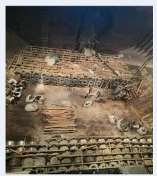
When the vessel arrived at the final discharge port, a considerable number of the coil outer packaging were found to have been affected by MAP spilled from the bagged cargo stowed above, and discharge at the previous port – as shown below. A large cargo claim was brought against the Owners.
