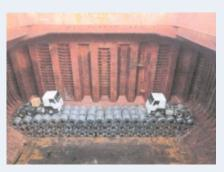
A five-hold geared bulk carrier loaded mixed stowage of bagged cargo, vehicles and steel products at China for offloading at Africa and Brazil. The Charterers' Pre-Stowage Plan had indicated to the Master that bagged cargo, vehicles and steel bars were planned to be loaded above steel coils. The Master did not raise any protest at this pre-stowage phase.
