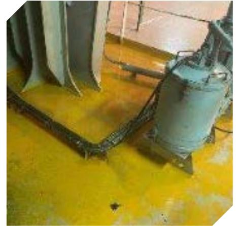
Hydraulic fluid accumulated in steering gear saveall
