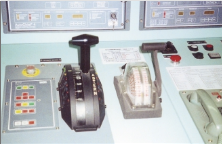
Bridge control main engines - a common factor in Sri Lanka accidents
