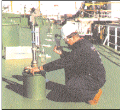
Closed cargo sampling in progress
