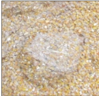
Inattention to the dangers of heat transfer from bunkers can leave cargo looking like this
