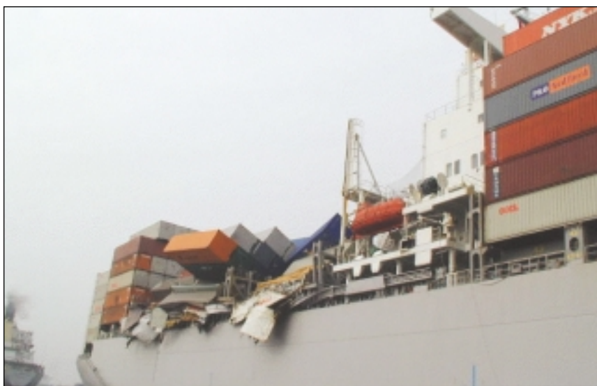
The design and size of large, modern containerships may be a factor in recent reported twistlock failures
