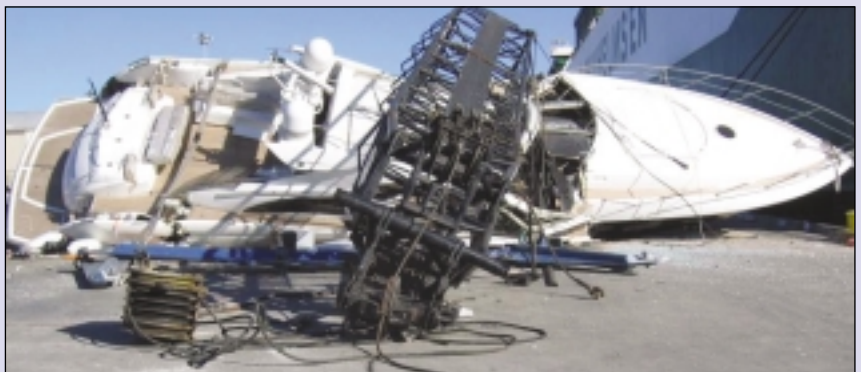
The above photograph shows the damage caused when a shore crane collapsed during discharge of a large yacht, which had been carried as deck cargo. The cause of the collapse remains under investigation.
