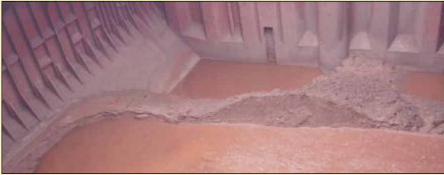
Free water is seen lying on top of liquefied ore fines
