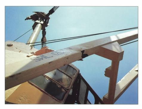
cranes' limit switches. If limit switches are being overridden, or are simply not working, intolerable pressure can be placed on the crane jib and other parts of the structure. The potential consequences are extremely serious.
