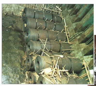
THERE are a number of ways to load steel cargoes. The picture below shows the correct way, while the photograph to the left shows what can happen when you do it the wrong way. No further commentary should be necessary.
