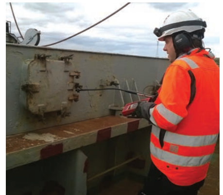
Ultrasonic hatch cover tests remain a significant loss prevention tool
