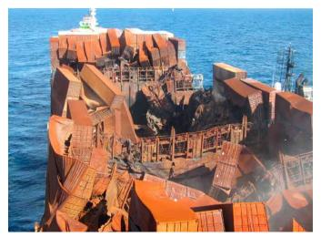
The aftermath of a container-related fire onboard a medium-sized container ship
